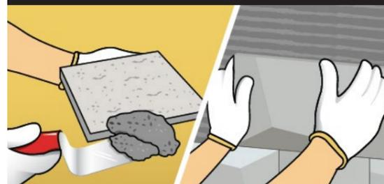
• Complete this step starting from the bottom of the wall & moving upwards: Apply a thick layer of mortar onto the back side of stone. Press and hold the stone firmly onto the mortared wall surface for a few seconds. Repeat this until the section is completed with stones. Use spacers and leveler if necessary to ensure a level arrangement.
