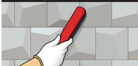
Once the stones are firmly affixed, clean the surface with a dry brush to clear the stones of any dust
