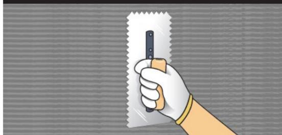
Apply a generous layer of mortar across the wall using the notched edge of a trowel, creating a "combed" surface pattern.
